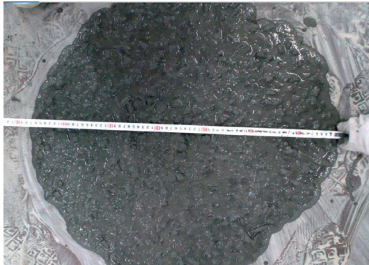
FIGURE 2: Slump flow of fresh SFRSCC.
