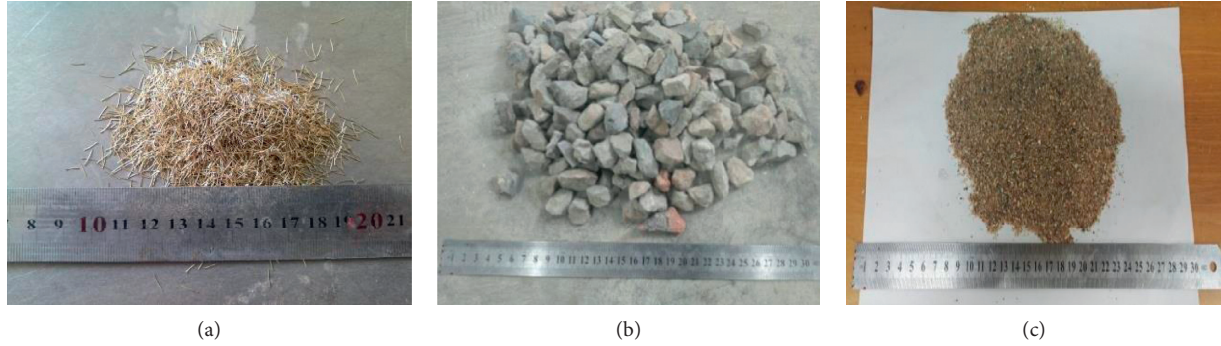
FIGURE 1: Materials used in this study: (a) steel fibres; (b) coarse aggregate; (c) sand.
