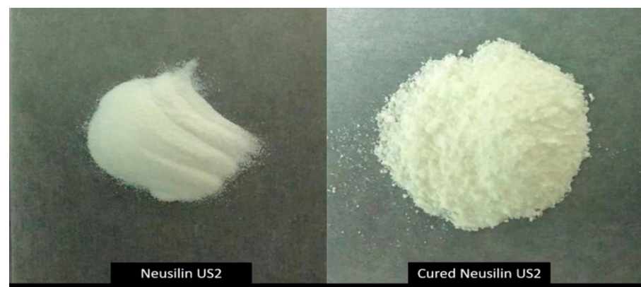
Figure 4. The inorganic silica material Neusilin US2 as uncured (purchased from the manufacturer) and cured (processed) form.
