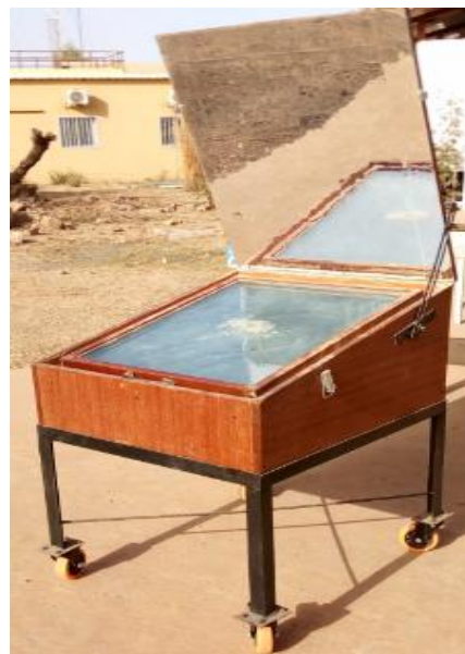
Fig. 1. Picture of the fabricated solar box cooker
