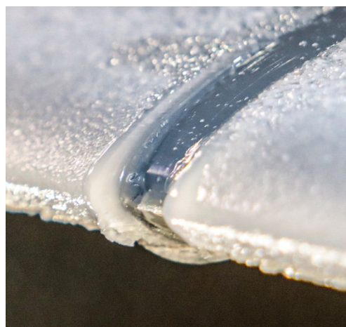
Figure 1. Chordwise cut into an ice shape that formed after 6 min of icing, shows how the entire leading-edge is covered by ice.
