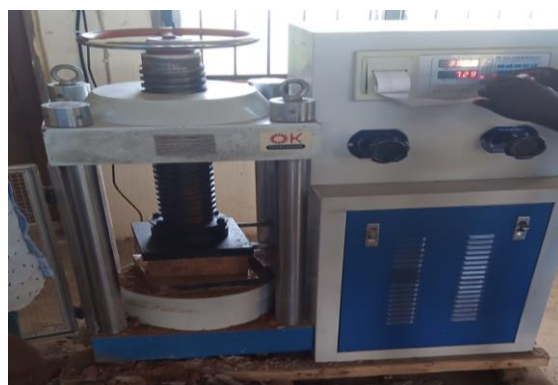
Fig. 6. Specimen being tested for compression
