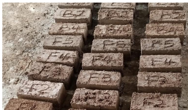
Fig. 4. Photograph showing freshly moulded block specimen
