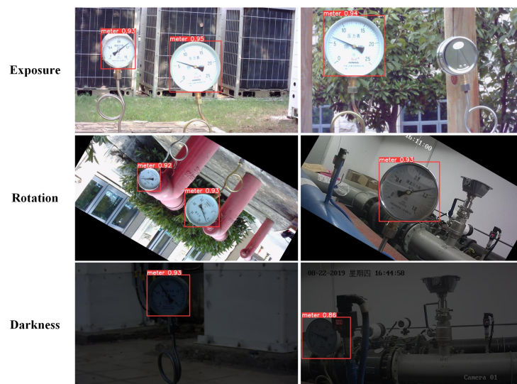
Figure 12. The dial detection results based on YOLOv8 under different challenging conditions.
