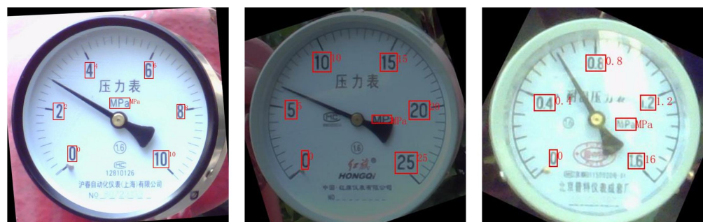
Figure 8. The recognition results of scale values and the unit.
