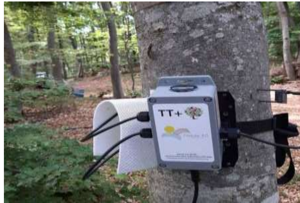
Fig. 7. Tree talker sensor used to monitor the tree
