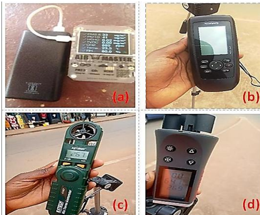
Fig. 2. The different devices needed for this study (a) Air analyser and charger, (b) Garmin type GPS, (c) Extech, (d) Anemometer
