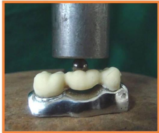
Fig. 13. Setup with temporary bridge and sphere prior to fracture testing
