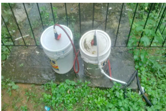
Fig. 1. The fabricated digesters
