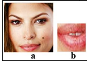
Fig. 7. a) Detected face after applying the Viola-Jones algorithm, b) Mouth Detection using Viola-Jones Algorithm
