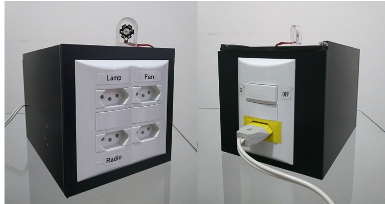
Fig 1. gBox: Electronic module to control home devices in the SE.
