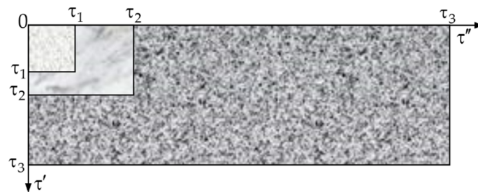
Figure 15. Schematic representation of set of integration regions in the points \tau = \tau_1, \tau = \tau_2, \tau = \tau_3 for g(\tau) = \tau^2 .
