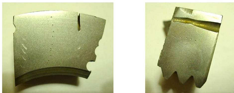
Figure 4. Hardness measurements at the site of the guide bar crack in both directions.
