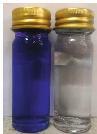
FIGURE 5: Comparison of colour between MB dye feed and filtrate water after adsorption process in batch column study.
