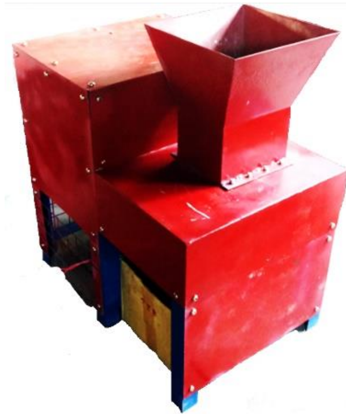
Fig. 3. Fabricated PET bottle shredding machine
