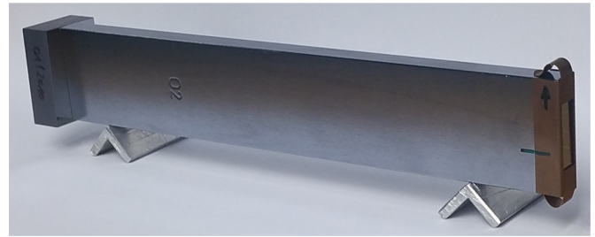
Figure 1. Close-up view of the silicon sample. The dimensions of the gauge-block-shaped body are 197 mm × 35 mm × 9 mm. At the back end face, the optically flat silicon reference plate is attached by wringing. At the front end face, a metal frame is softly clamped onto the gauge block to mask edge damage and to facilitate the edge detection within the interference pattern recorded by the camera.
