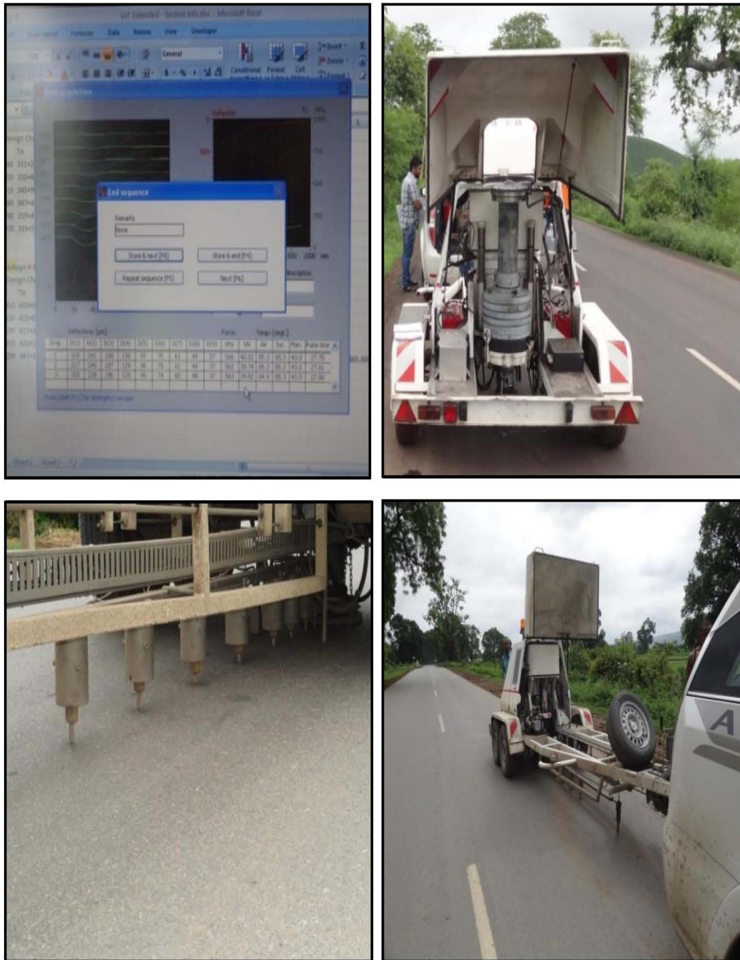
Fig. 5. FWD test photos
